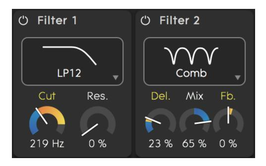
The low-pass, high-pass, band-pass and notch filters have the following parameters:
