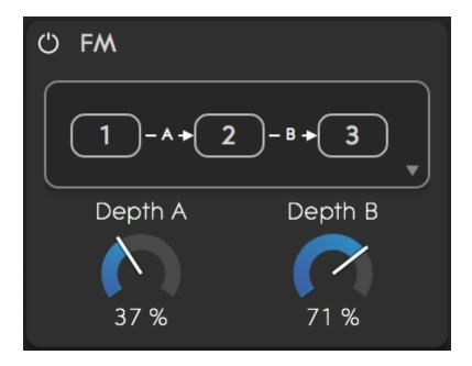
Note: FM synthesis is available only for the waveform oscillators, not for the Sample Playback modules in Equator.
