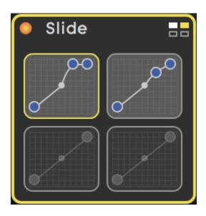
For each source, you can add points along the transfer curve by doubleclicking on the curve. This can be used to create unipolar responses as well as more complex transfer curves. To remove a point, just double-click on the one that needs removing.
