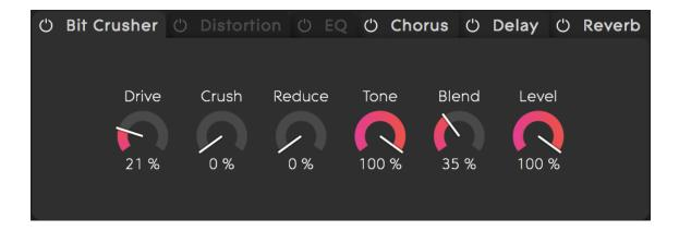
Bit crushing literally reduces the bit depth of a digital signal (for example, from 24 to 16 or even 8 or fewer bits), often to produce an intentionally "lo-fi" sound reminiscent of vintage digital synths, drum machines, and/or video games. Equator's Bit Crusher also performs sample rate reduction, giving you still more control over the lo-fi character.
