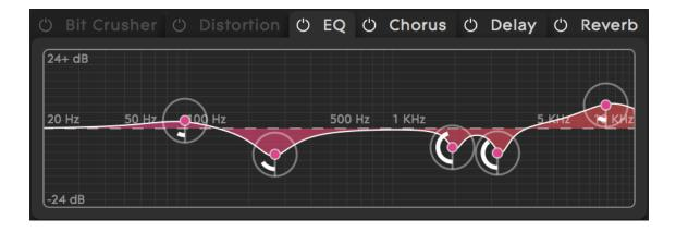
The EQ section is a five-band parametric equaliser. Each band has the following parameters:
