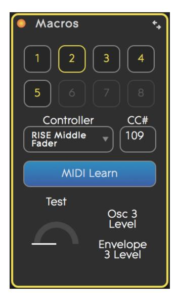
The Switch View button (in the top right-hand corner of the RISE Controls section) displays the assignable macros. Macros can be assigned to MIDI CC messages of any external MIDI controller connected to Equator. Macros default to these settings:
