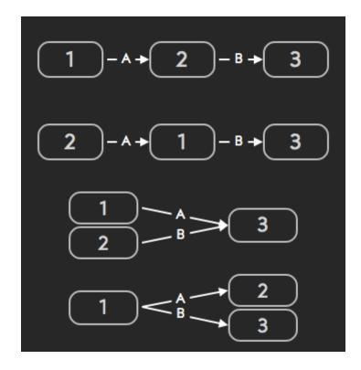
Note that each arrow is labeled with a letter A or B. You can control the depth (intensity) of each modulation segment using the corresponding Depth A and Depth B dials.
