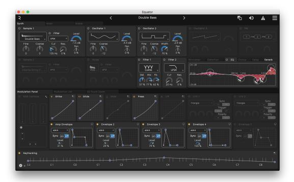
Above is the main view of Equator, showing the Synth Panel at the top half of the screen and the Modulation Panel at the bottom half of the screen.
