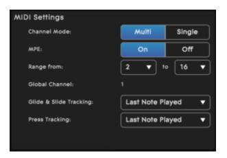
You can select channel mode and customise behaviour of the GRAND on the MIDI Settings Panel. This section can optimise the GRAND with third-party hardware and software synths. The selection of Channel Mode (Multi Channel or Single Channel) and the activation of MPE (Multidimensional Polyphonic Expression) (On or Off) is the primary function of this section. Other features such as channel range and **Glide** and **Press** Tracking are detailed below.
