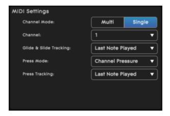
In Single Channel Mode the RISE transmits all MIDI data on a single MIDI channel only. This makes it compatible with mono-timbral synths. Pitch bend, channel pressure, or Slide (MIDI CC 74) messages will apply to all notes held.
