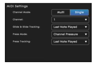
In Single Channel Mode the GRAND transmits all MIDI data on a single MIDI channel only. This makes it compatible with mono-timbral synths. Glide and Press messages will apply to all notes held.
