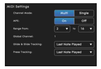
You can select channel mode and customise behaviour of the RISE on the section of the MIDI Settings Panel called "MIDI Settings." This section can optimise the RISE with third-party hardware and software synths. The selection
