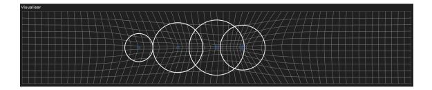
The **Visualiser** is a real-time graphical representation of the **keywave surface** of the RISE. As you play on the **keywave surface**, the **Visualiser** responds to the Five Dimensions of Touch: **Strike** (translucent blue circle), **Press** (circular white outline and "warping" of the grid background), **Glide**, **Slide**, and **Lift**. Experiment with the **Visualiser** by making any gesture on the **keywave surface**.
