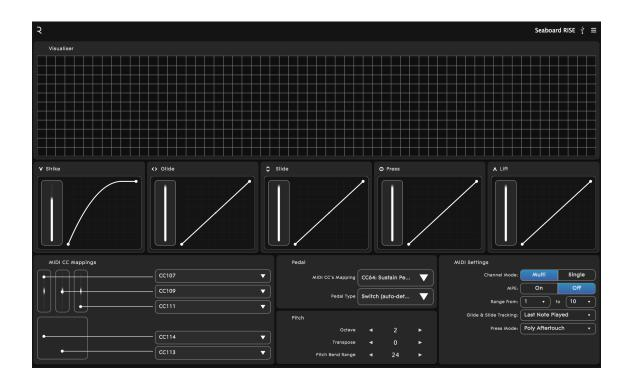
**ROLI Dashboard** is an application that lets you both customise the internal settings of the Seaboard, and modify the signals being sent by your instrument. The settings that can be edited from **ROLI Dashboard** depend upon
