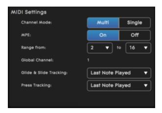
Selecting Multi Channel Mode and turning MPE "ON" optimises the GRAND with any other hardware or software that supports MPE.
