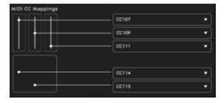
You can map MIDI CC messages to the **Glide**, **Slide**, and **Press** Touch Faders as well as the X and Y axes of the XY Touchpad. Click the arrows to access a pull-down menu of possible MIDI CC mappings. The RISE will retain these mappings even after it is powered off.
